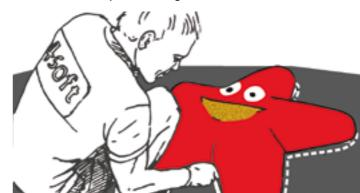
Spread one or two component glue evenly directly on SBR-Take care about upper side of component to avoid stain of glue on it!
