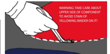
Screed and compress your final EPDM coat around your 3D component. Cartridges or salami. For example Proline T44 or Extrem FIX.
