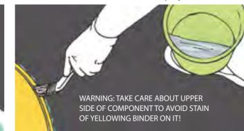
Spread and compress properly your final EPDM coat around the component.
